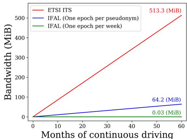
Fig. 10. IFAL vs. ETSI ITS: Cellular bandwidth requirements
